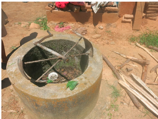
Fig. 4. Broken mixture and stirrer.
